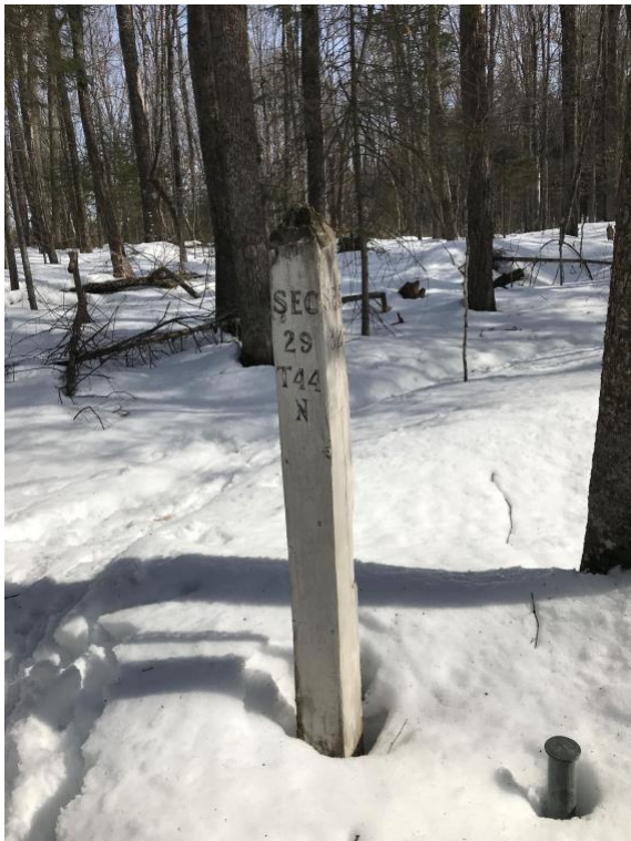
An old Public Land Survey System township corner marker alongside a modern National Geodetic Control marker near the crest of the Laurentide divide just east of Diamond Lake.
